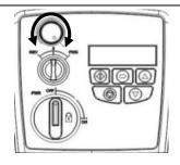
The potentiometer will control the motor shaft rotational speed.
