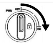
Switch the mains power on to the unit using the built in isolator switch on the front panel.
